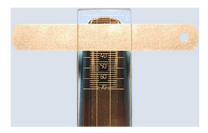
To determine the contact point of a mouthpiece, place a reed correctly on the mouthpiece, and place a thin piece of paper (unless you have one of these fancy shims!) between the side rails and the reed table.
