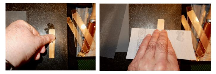
Then sand the table of the reeds over 3200 Micromesh, followed by 6000 Micromesh sandpaper. This is an abrasive that was developed for polishing commercial aircraft windows—they go up to 12,000, which is too fine for reed work but excellent for polishing mouthpieces after re-facing. 600 grit commercial wet/dry sandpaper from a hardware store works well, but I'm a fanatic. If you finish with 6000 Micromesh the table of your reed will be as smooth as glass.
